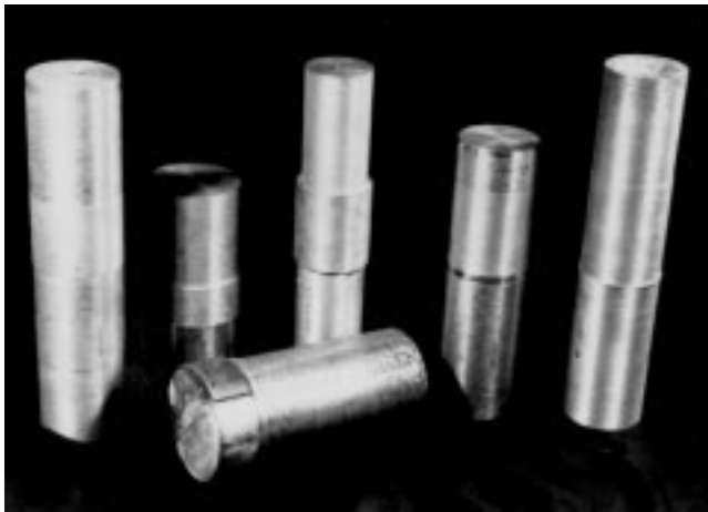
Fig. 1 LM6/LM25-SiCp composites cylinders (75 mm diam by 170 to 270 mm long) used as work pieces
